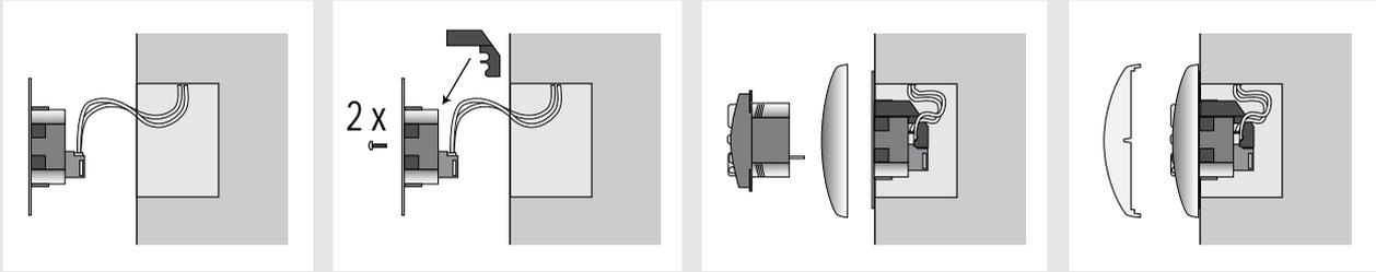
Connect the wires to the terminals of the connecting bracket in accordance with the terminal layout (chapter 2.2).
