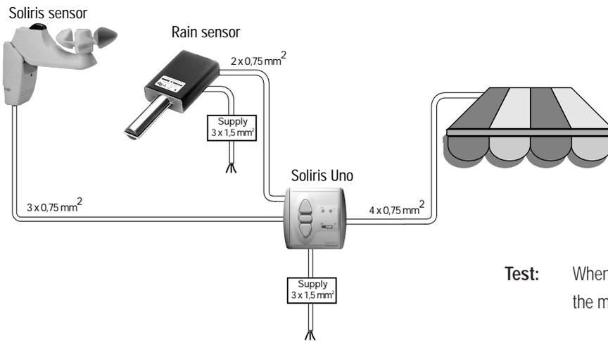
**Test:** When operating power has been connected, the direction of the motor can be tested using the ▲ and ▼ buttons.
