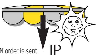
The awning goes to the intermediate position IP (see 4.2) or to its down end limit position if no intermediate position has been memorised.
