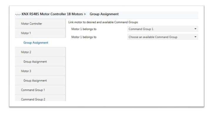
The settings for the group assignments are exemplarily described on "Motor 1". Depending on the number of motors selected in the menu "Motor Controller", the settings have to be done for all further motors (motor 1....18).
