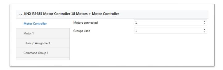
With this menu index card it can be stated how many motors are connected on the Motor Controller and how many command groups shall be used for the connected motors.
