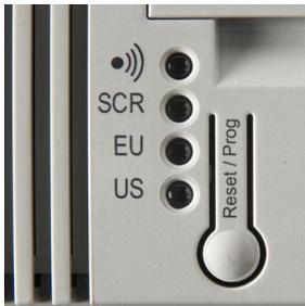
The “US”-LED blinks regularly when the mains (24 V) and the KNX bus voltage are connected actively on the device. The device is ready for operation when the “US” LED blinks.
