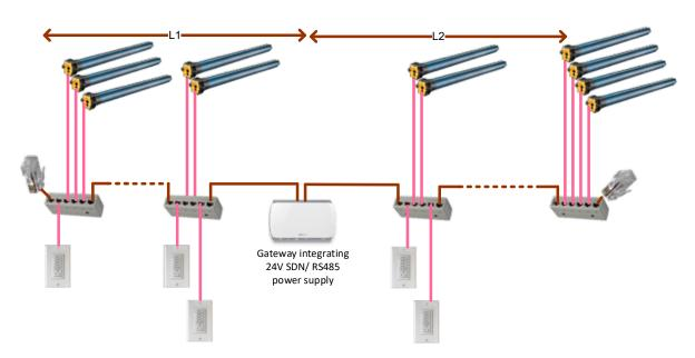
L1: the current needed by powered devices is 240mA. Chart -> max. possible 500 m.
