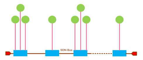
SDN bus: The maximum length cannot exceed  $1200 \, \text{m} / 4000 \, \text{ft}$  and refers to the controller documentation. Junction: passive must be used.
